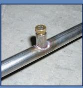
1/2" stainless steel pipe with 0.02 gpm anti-dripping valve
